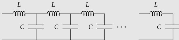
What resistance  $R$  placed at the end (in parallel with the last capacitor) makes the cable look like an infinitely long LC cable?
