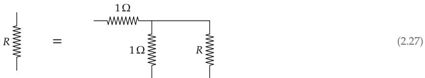
The next step in finding  $R$  usually invokes the parallel-resistance formula: that the resistance of  $R_1$  and  $R_2$  in parallel is
