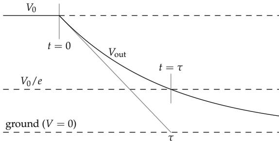
After one time constant  $\tau$ , the capacitor voltage falls by a factor of  $e$  toward its final value—here, from  $V_0$  to  $V_0/e$ . The  $1/e$  time is our first interpretation of the time constant. Furthermore, if the capacitor voltage had decayed at its initial rate (just after  $t = 0$ ), it would have reached zero voltage after one time constant  $\tau$ —the second interpretation of the time constant.
