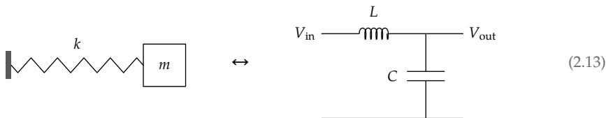
In the circuit, the voltage source—the  $V_{in}$  on its left side—supplies a current that flows through the inductor (a wire wrapped around an iron rod) and capacitor (two metal plates separated by air). As current flows through the capacitor, it alters the charge on the capacitor. This “charge” is confusingly named, because the net charge on the capacitor remains zero. Instead,
