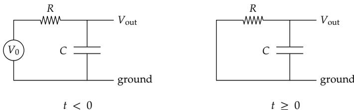
The capacitor discharges through the resistor, and its voltage decays exponentially:
