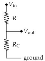
In the  $RC$  circuit, thought of as a voltage divider,
